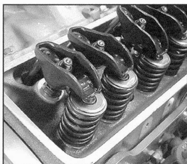
3 If both rocker arms for #1 cylinder are parallel as shown here (valves closed) with the timing index line on the balancer aligned with the "0" on the timing tab, the engine is at #1 TDC on the compression stroke.
